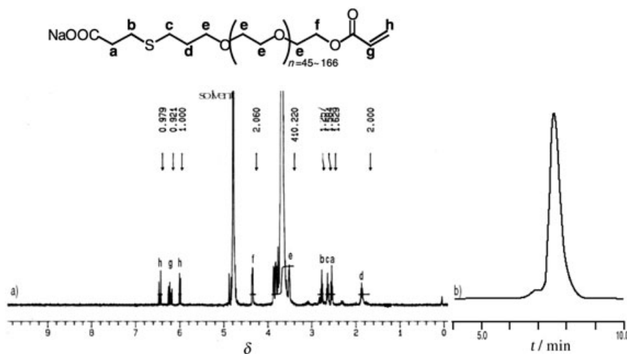
Figure 2. a) ^1\text{H NMR} spectrum, and b) SEC chromatogram of HOOC-PEG-acrylate.
